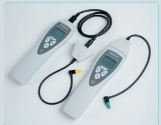
The OtoRead™ allows the use of extension cables and can thus be used handheld or can lay beside the patient.
